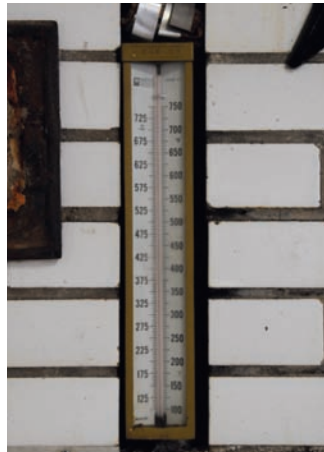
This thermometer is built into the bricks of the oven.
